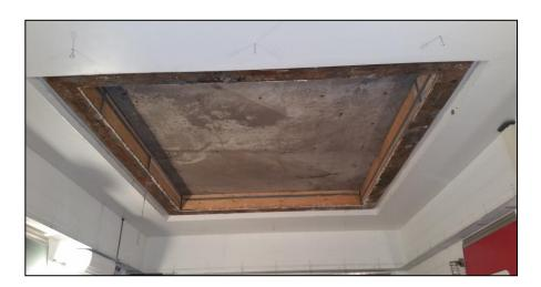
**Receive Room View of Test Specimen Installation**
