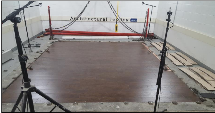
Source Room View of Test Specimen Installation
