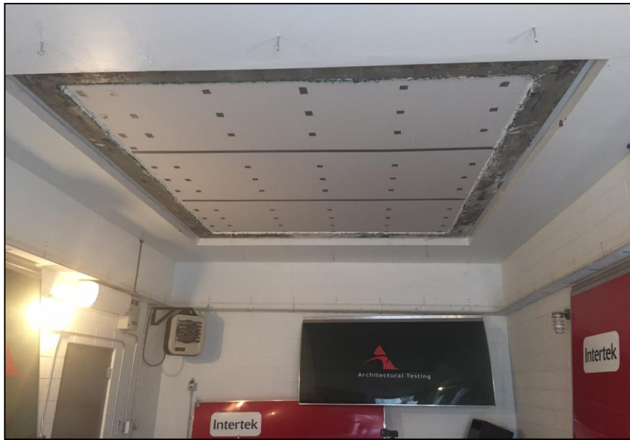
Receive Room View of Test Specimen Installation
